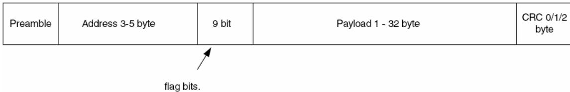
**Figure 19.** Enhanced Shockburst data packet
